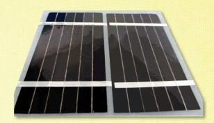
Flexible CISe solar foil may be integrated into customized modules for power generation in a wide spectrum of ground and space applications.
